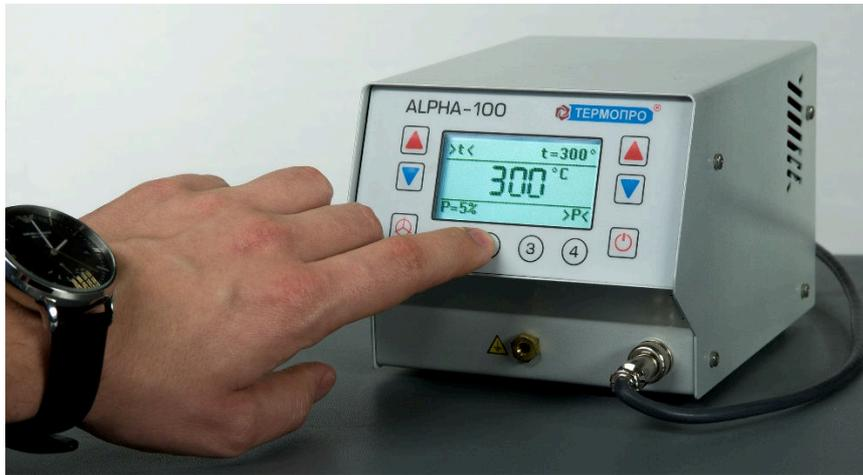
*Pic. 7 A store of temperature settings in memory cell for a further fast change.*
