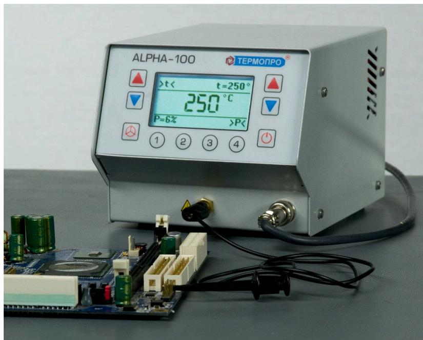
*Pic. 8 Connection with unit for equipotential soldering.*
